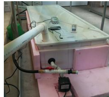
Water tank with pump and bubbler
